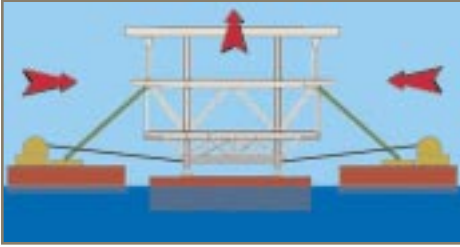
Fig. 2. When lift winches are engaged, the two lift barges are pulled toward the transport barge. As they draw together, the booms rotate on their heel pins, thereby increasing the angle of the booms and raising the deck. Once in position, the deck is lowered by releasing tension on the cables.
